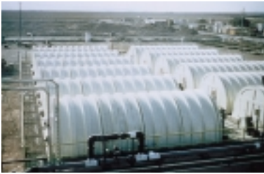
RBCs are installed around the world because of their simple and economical operation.
