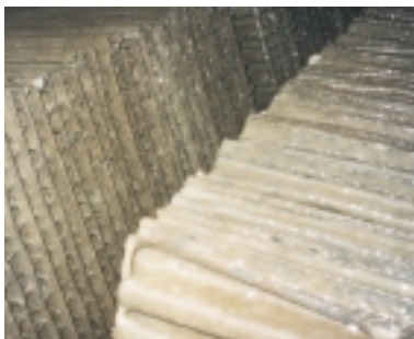
Biomass is evenly distributed over the media surface.
